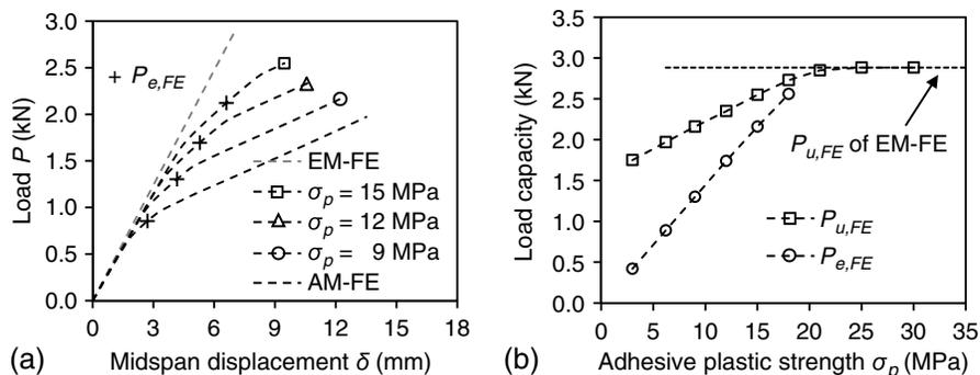
**Fig. 11.** Effect from FE modeling of adhesive plastic strength ( $\sigma_p$ ) on (a) load–displacement ( $P$ – $\delta$ ) behavior; and (b) load capacities ( $P_{e,FE}$  and  $P_{u,FE}$ ).
