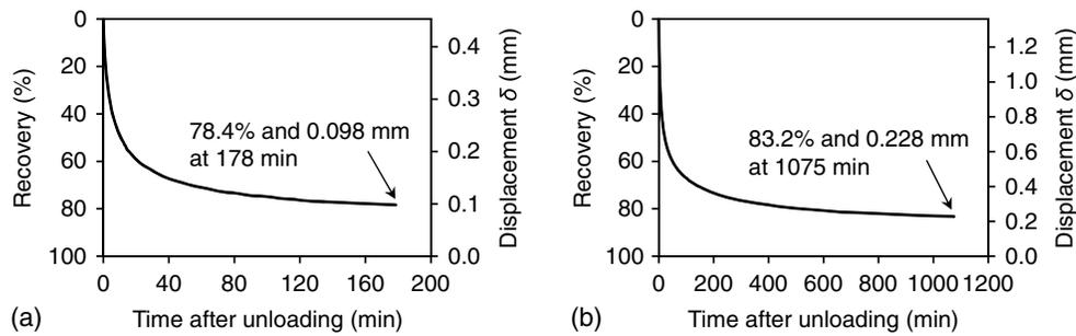
**Fig. 9.** Recovery of residual midspan displacement ( $\delta$ ) with time (Specimen AC-2): (a) after unloading at 0.85 kN; and (b) after unloading at 1.25 kN.
