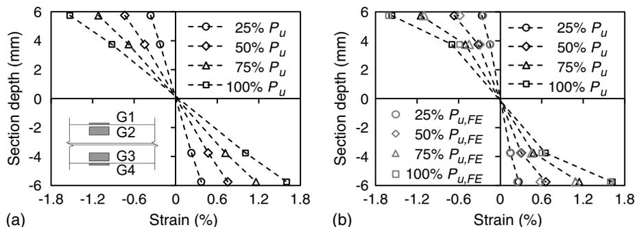
**Fig. 8.** Strain distribution along section depth: (a) Specimen EM-1; and (b) Specimen AM-1.
