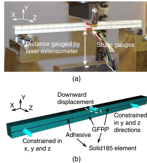
**Fig. 4.** Layered beam specimens under three-point bending: (a) experimental setup; and (b) FE modeling.
