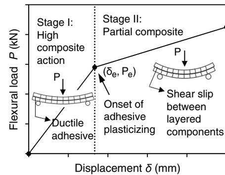
Fig. 1. Design concept for realizing nonlinear load-deformation response in beam structures.
