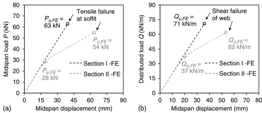
**Fig. 13.** Load-displacement responses of the GFRP built-up section beams under (a) midspan point load  $P$ ; and (b) uniformly distributed load  $Q$  (refer to Fig. 12 for cross section and span dimensions).
