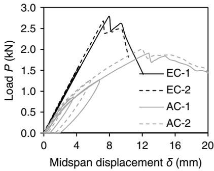
**Fig. 7.** Load-displacement ( $P$ - $\delta$ ) response of the beam specimens under load-unload-reload cycles.
