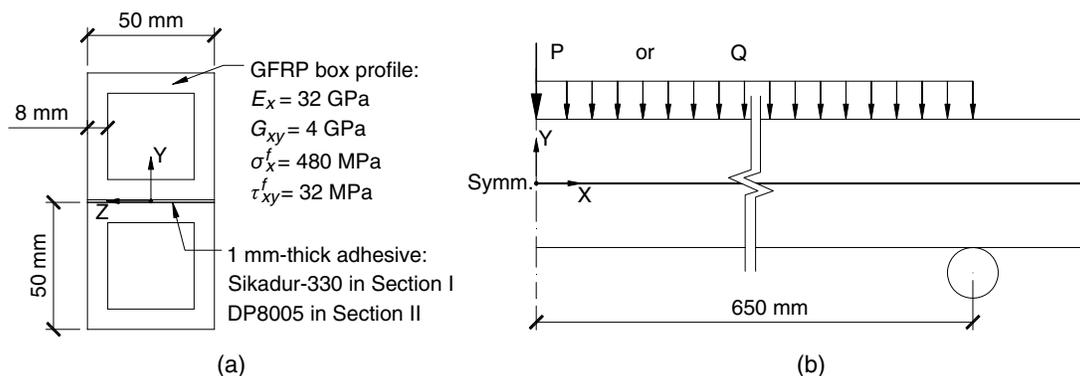
**Fig. 12.** GFRP built-up section beams: (a) cross-section dimensions and material properties ( $E$  = elastic modulus,  $G$  = shear modulus,  $\sigma^f$  = tensile/compressive strength, and  $\tau^f$  = shear strength); and (b) span dimension and load scenarios.
