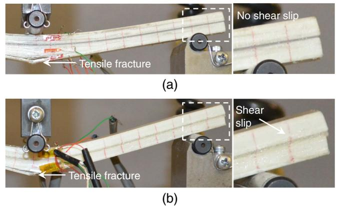
Fig. 6. Deformations and failure modes: (a) specimens with epoxy adhesive; and (b) specimens with acrylic adhesive.
