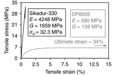
**Fig. 3.** Typical tensile stress-strain curves of adhesives Sikadur-330 and DP8005 and their material properties ( $E$  = elastic modulus,  $G$  = shear modulus,  $\sigma_u$  = ultimate strength, and  $\sigma_p$  = plastic strength).
