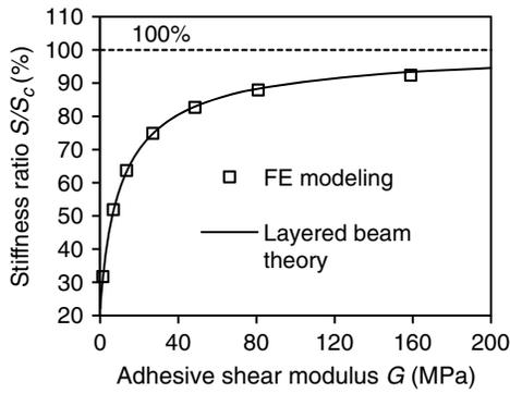
**Fig. 10.** Effect of adhesive shear modulus ( $G$ ) on stiffness of the layered beam from layered beam theory and FE modeling ( $S_c$  = stiffness when full composite action is present).
