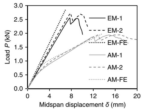
Fig. 5. Load-displacement ( $P$ - $\delta$ ) response of the beam specimens under monotonic loading.
