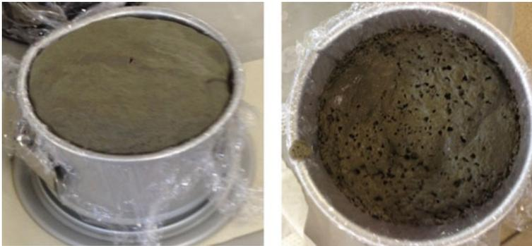
**Fig. 1** Foam concrete with (left) and without (right) foam stabilizer during plastic state
