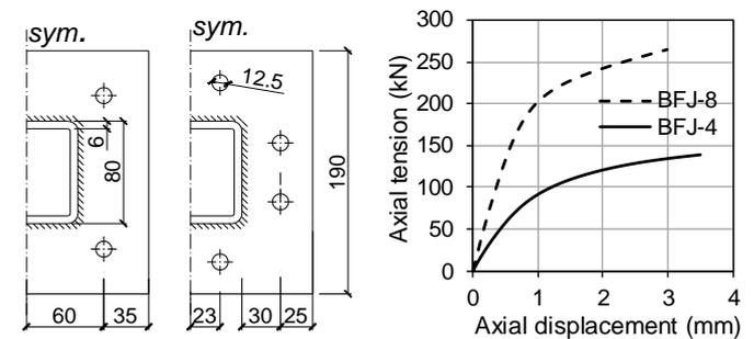
Fig. 6: Dimensions (units in mm, left) and tensile load-displacement behaviour (right) of BFJs
