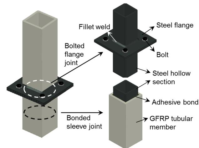
Fig. 1: Proposed column-splice connection for tubular GFRP members
