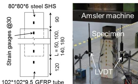
Fig. 2: Geometries of BSJ specimens (left, units in mm) and test setup (right)
