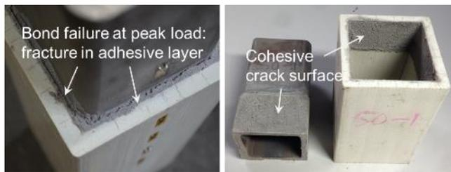
Fig. 3: Cohesive failure of BSJs
