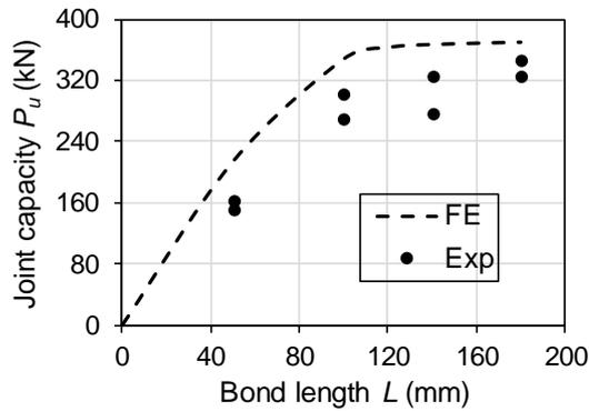
Fig. 4: BSJ axial joint capacity versus bond length
